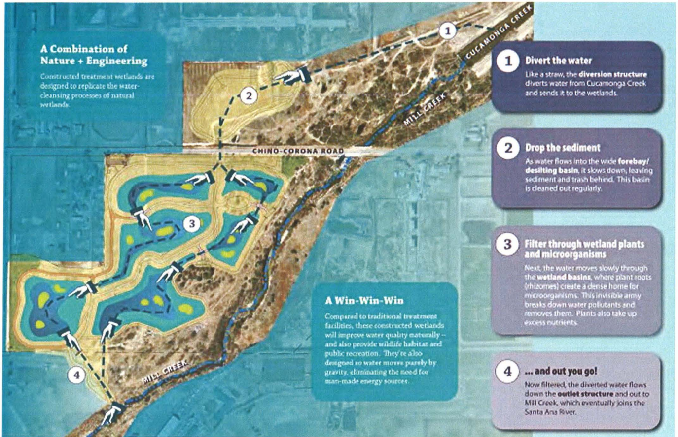
FIGURE 3. MILL CREEK WETLANDS' UNIQUE WATER QUALITY TREATMENT DOUBLES THE EFFECTIVENESS OF A TRADITIONAL, SINGLE-FUNCTION PROJECT
